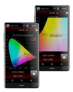
SS04B can measure illuminance and chromaticity of a light source at the same time. Chromaticity is evaluated according to CIE 1931 and CCT-Duv diagrams.
