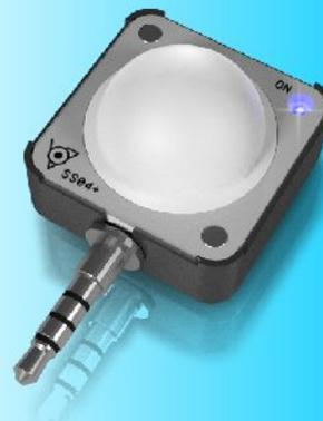
SS04 is a device designed for measurements of illuminance based on a high accuracy photosensor with sensitivity matched to the human eye. SS04 can easily be applied to a smartphone and can turn it into a professional instrument. You can use SS04 to take measurements on 3D objects or, with the supplied light shield, on flat objects. The sensor has a wide measurement range and can capture very short light impulses such as flash strobes.
